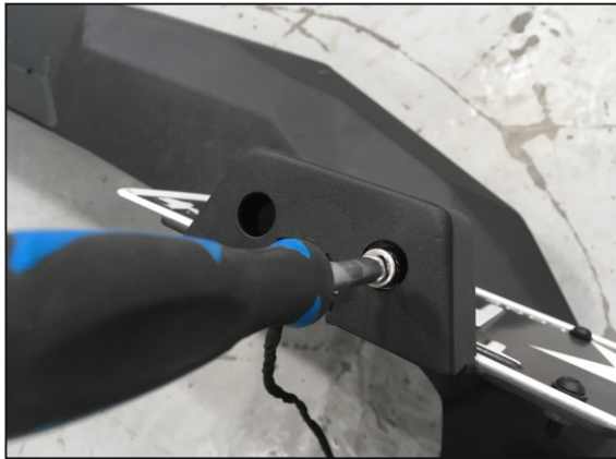
19. Fix license plate lights using OE fitting fit. Be careful, do not damage
