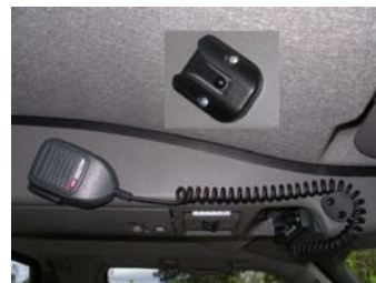
Install microphone clip on acute angle
