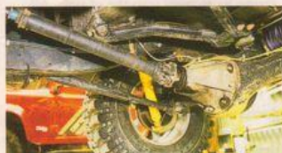
TOP: New guard due soon to suit bespoke engine position ABOVE: Off-the-shelf 200Tdi propshafts fit BELOW RIGHT: Ladders on rear
