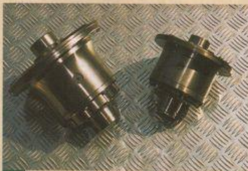
1 Rover diff-centre is on the right with the much larger (and stronger) Salisbury unit shown on the left
