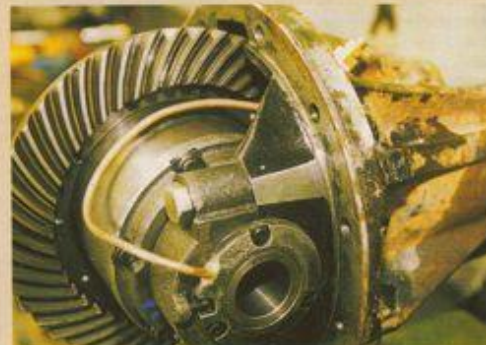
7 Seal housing that actuates locking action is shown here, together with air supply pipe. Make sure this pipe doesn't foul on any of the cogs
