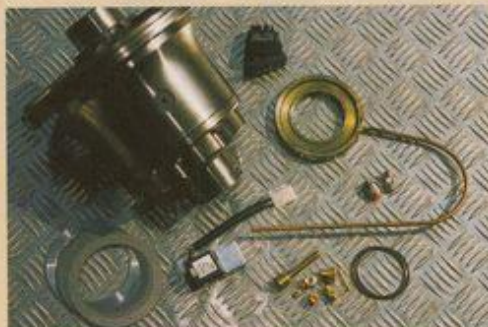
2 ARB diff-centre fitting kit with switch and compressor switch solenoid. Instructions run to 40 pages so this is no lunchtime fix – you have been warned
