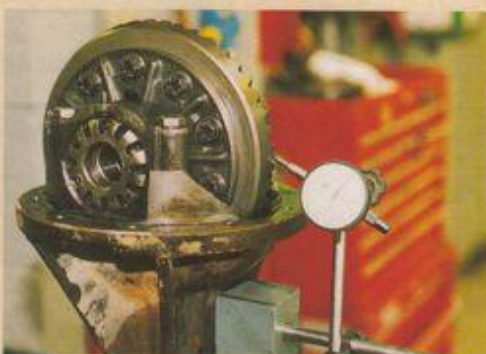
5 Setting up the preload with the dial-gauge. This needs to be spot on, so refer to a workshop manual for correct figures. Don't try to guess
