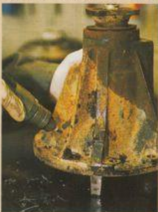
4 Drill diff-case on the opposite side to where the crownwheel runs and tap hole to take the airline union required to initiate diff-lock. Hole should be drilled on the top of casing and not on the bottom...
