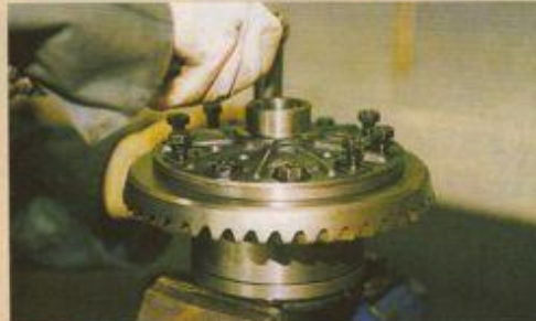
3 Original crownwheel being fitted to new ARB diff-centre. Bolts should be tightened diagonally, 'loctited' and torqued down to correct figures. It may be necessary to warm crownwheel on a slow heat. Do not be tempted to use direct heat (oxy-acetylene torch), this will affect the tempering and hardness of the gear
