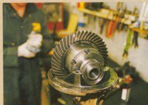
6 Fitting new diff-bearings is a wise move at this stage of proceedings, could save time and money later
