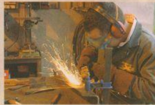
LEFT TO RIGHT: Bumper in its raw state; Matthew Cook welds the separate pieces together; He then grinds it, tidying up the welds in the process
