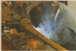
LEFT TO RIGHT: Bumper in its raw state; Matthew Cook welds the separate pieces together; He then grinds it, tidying up the welds in the process
