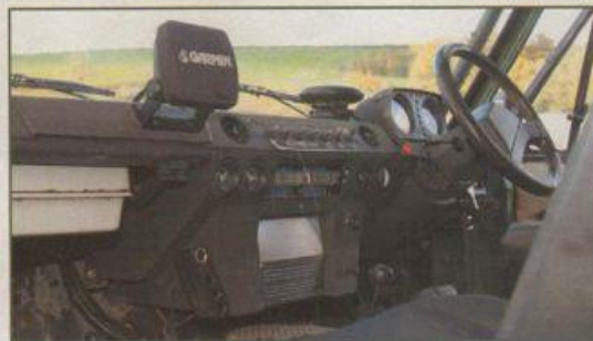
Working cabin area: GPS for navigation, and all switches and fuses are easily accessible
