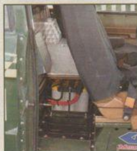
Twin batteries are situated behind the seats
