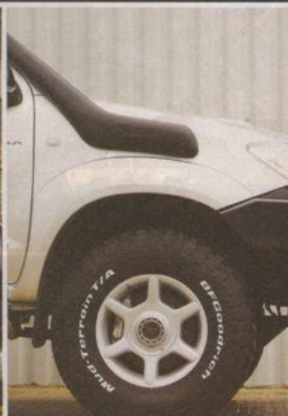
The Safari Snorkel is the only modification under the Hilux's bonnet
