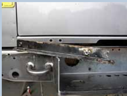
Cut and trimmed rear body mounting bracket
