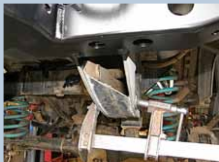
New side rails assembled and welded in-situ
