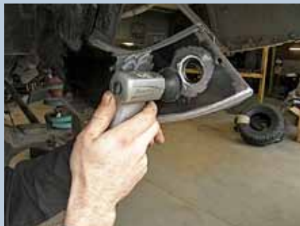
Every inch of weld site is carefully prepared
