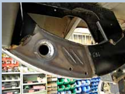
... two long puddle-welded slits add strength
