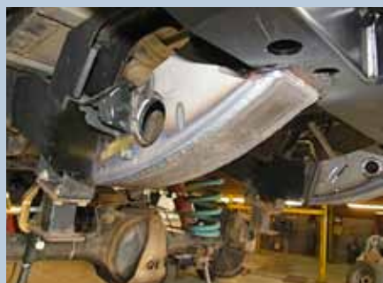
Side rails seam-welded on every edge...
