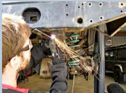
Plasma cutter slices through steel cleanly
