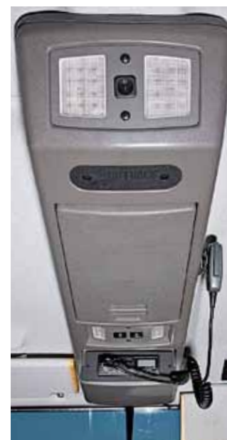
Roof pod houses powerful LED lights, CB and map compartment
