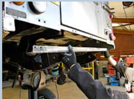
The body mounting bracket will be modified
