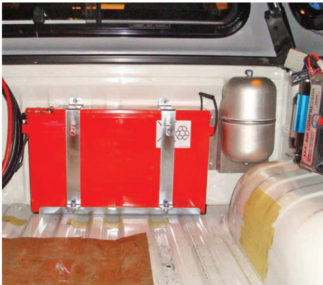
Bottom left: Custom fabricated fixing brackets hold the ARB compressor and air tank in place
