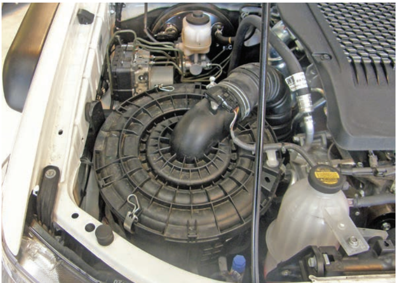
Left: Air filter all sealed up and sitting pretty in engine bay
