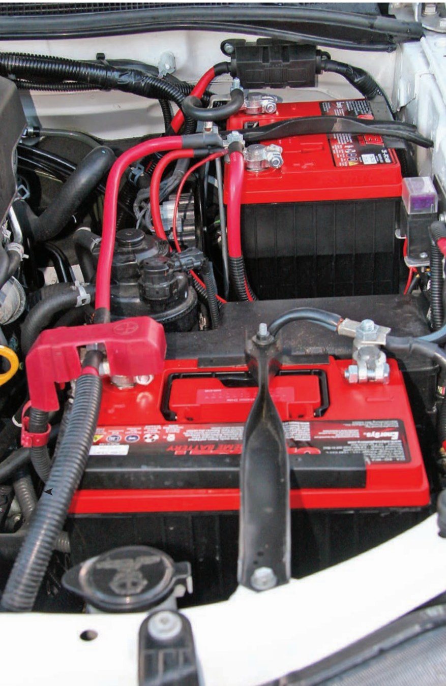
Left: Odyssey PC1400 batteries give plenty of power on start up while a Merlin split charge system looks after fridge contents
