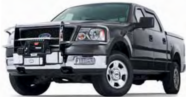
Ford F-150 equipped with Stainless Steel Trans4mer Grille Guard, Brush Guards, Winch Carrier, PowerPlant winch, SST Carrier Cover, Angled Light Bar.
