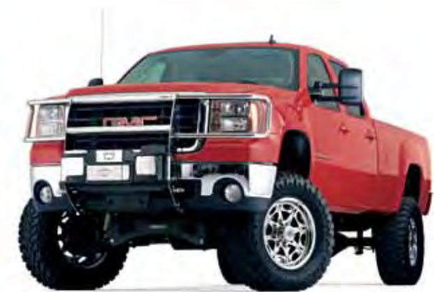
GMC Sierra HD equipped with Stainless Steel Trans4mer Grille Guard, Brush Guards, Winch Carrier, M15000 Winch, and SST Carrier Cover.
