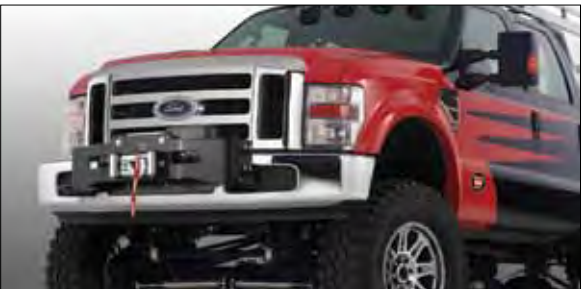
Gen II Trans4mer Mounting Kit, with 16.5ti winch (Mounting Kit includes winch tray and mounting brackets).
