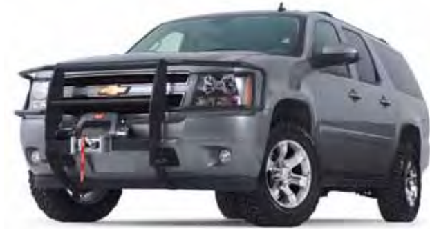
Chevrolet Suburban equipped with black powder-coat finish Trans4mer Grille Guard, Brush Guards, Winch Carrier, and 9.5cti Winch.
