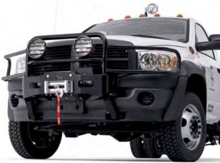
2010 Dodge HD equipped with WARN Gen II Trans4mer Mounting Kit, Grille Guard Tube (tall version), Headlamp Guards, and Light Bar
